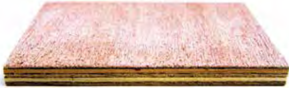
Figure 39. Typical plywood showing okoume veneer on its face. Source: EIA
