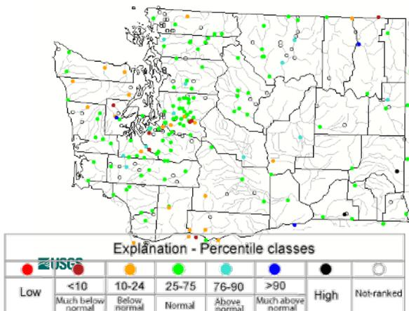
Figure 5: July average streamflows for WA from [USGS](#).
